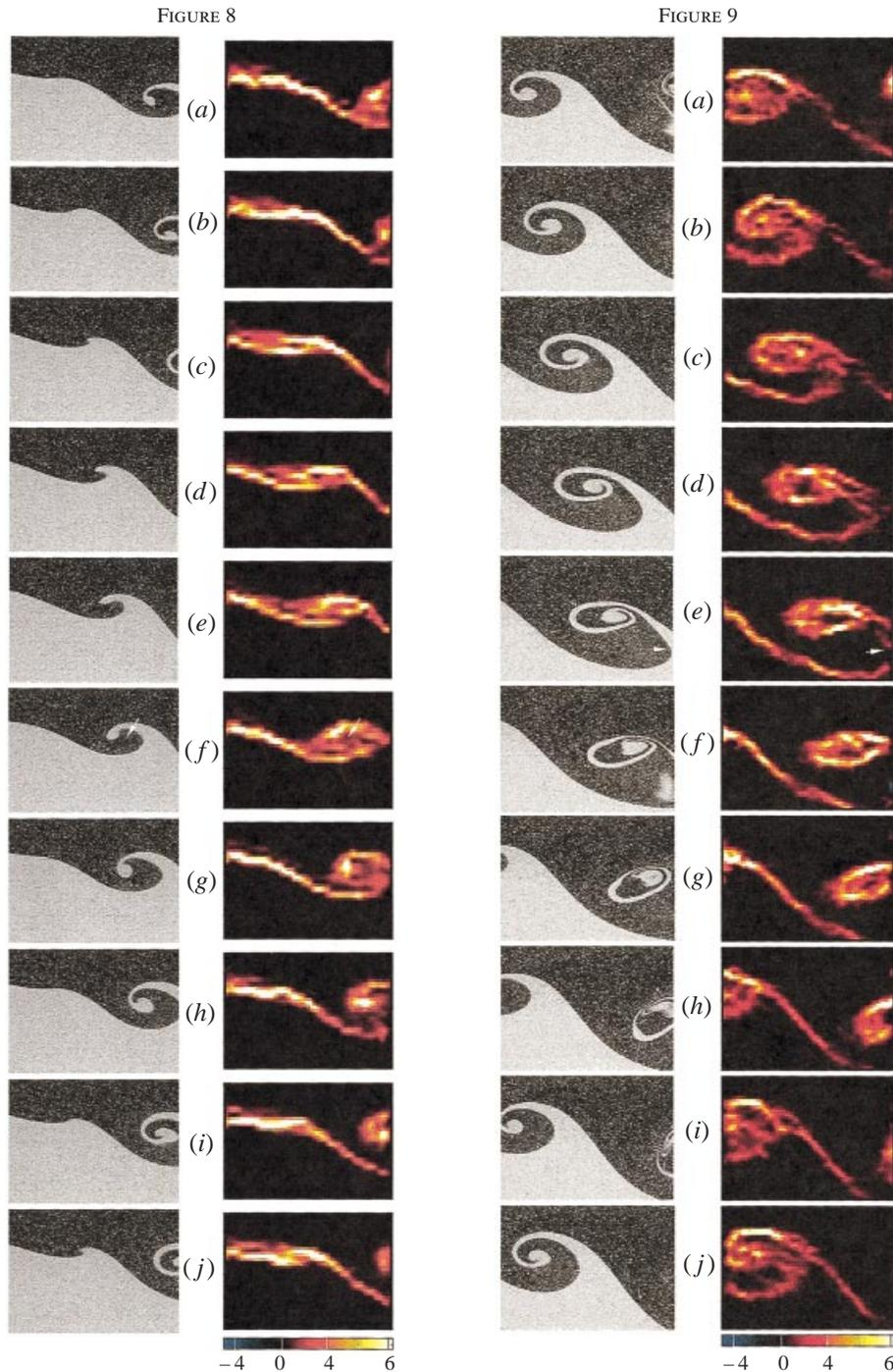
FIGURE 8. Image (left-hand column) and vorticity (right-hand column) sequence at onset of instability for intermediate acceleration case. Each frame is a 0.1 s average at intervals of 0.5 s. Physical dimensions of the images are approximately 10 cm  $\times$  7.5 cm. Vorticity scale is shown with the colourbar with units of 1/s.
